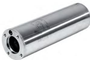
Canned stator with external shell and flanges made in AISI 304L stainless steel. The stator has 24 slots for better elasticity and regularity of operation. Class F double insulated copper wire. Thermal protection included in the motor from 0,5 HP to 1,5 HP in the 50 Hz version, from 0,5 HP to 1 HP in the 230 V - 60 Hz version.
