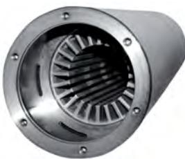
The stator is rewirable type and it's inserted in an AISI 316 stainless steel outer shell. In the standard version the windings are made in copper insulated by PVC (PE2+PA on 300 HP and 340 HP). On request it's available the PE2+PA windings for special applications such as the use with a variable frequency drive.
