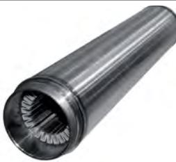
The stator is rewirable type and it's inserted in an AISI 316 stainless steel outer shell (on request AISI 904). In the standard version the windings are made in copper insulated by PVC. On request it's available the PE2+PA windings for special applications such as the use with a variable frequency drive.
