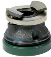
Kingsbury type thrust bearing unit consisting of tilting pads made of highly-resistant stainless steel and machined by Tesla using the spherical lapping process. From 0,5 HP to 1.5 HP: 2000N (450 lbf) (3000N (700 lbf) in the 1.5 HP 60 Hz version)
