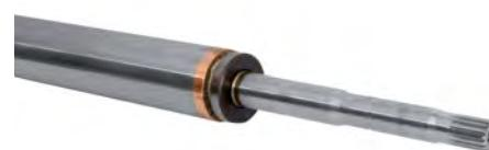
The stator is rewirable type and it's inserted in an AISI 304 stainless steel outer shell (on request AISI 316 or AISI 904). In the standard version the windings are made in copper insulated by PVC. On request it's available the PE2+PA windings for special applications such as the use with a variable frequency drive.
