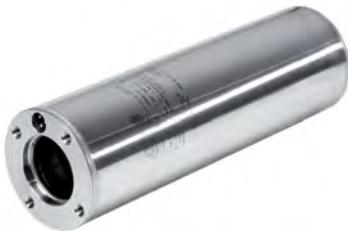
Canned stator with external shell and flanges made in AISI 304L stainless steel. The stator has 24 slots for better elasticity and regularity of operation. Class F double insulated copper wire.
