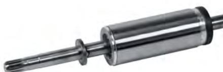
Shafts with end part made of stainless steel AISI 304 with a special process of surface hardening and polishing of the working area of the bushes. Squirrel-cage rotor made in aluminum.
