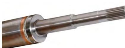
Shafts made of stainless steel with end part according to 8" NEMA norms. Squirrel-cage rotor made in copper. In the standard version the motor is equipped with a ceramic/carbon mechanical seal. On request it's available the silicon carbide (SiC/SiC) mechanical seal. On request the motor can be equipped also with a lip seal (granting the IP 68 insulation).
