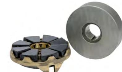
Mitchell type thrust bearing unit consisting of tilting pads in stainless steel covered by rubber and stainless steel disc. From 200 HP to 340 HP:
