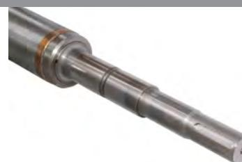
Shafts made of stainless steel with end part with key coupling. Squirrel-cage rotor made in copper. In the standard version the motor is equipped with a ceramic/carbon mechanical seal. On request it's available the silicon carbide (SiC/SiC) mechanical seal. On request the motor can be equipped also with a lip seal (granting the IP 68 insulation).
