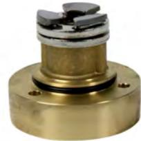
Kingsbury type thrust bearing unit consisting of tilting pads made of highly-resistant stainless steel and machined by Tesla using the spherical lapping process.
