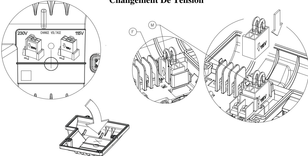
**MISE EN PLACE DU CONVERTISSEUR DE TENSION**
