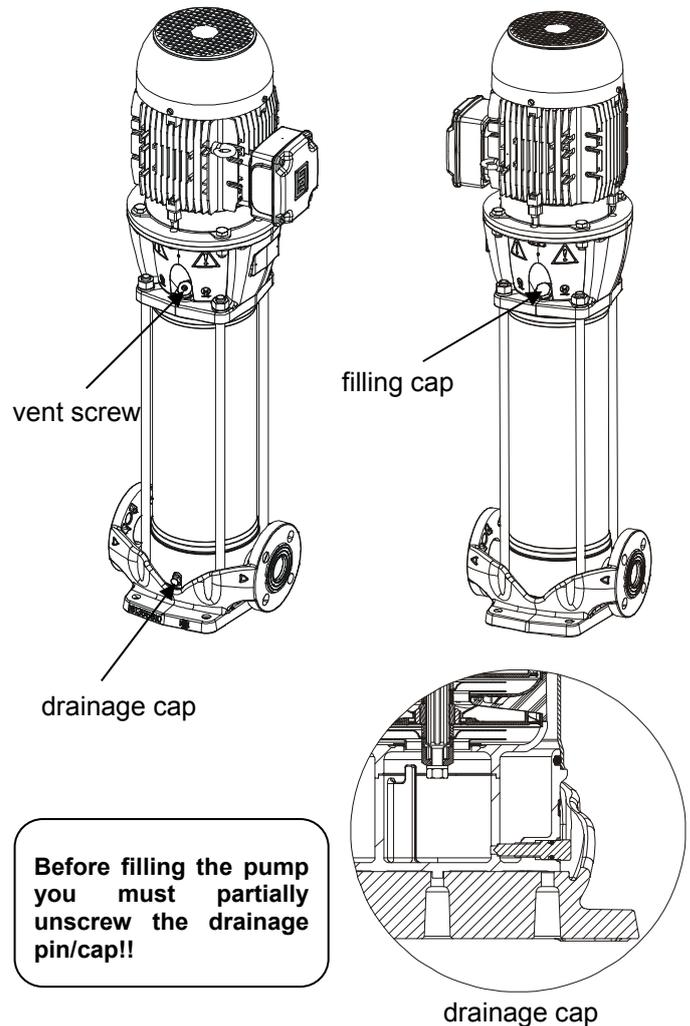
**Before filling the pump you must partially unscrew the drainage pin/cap!!**
